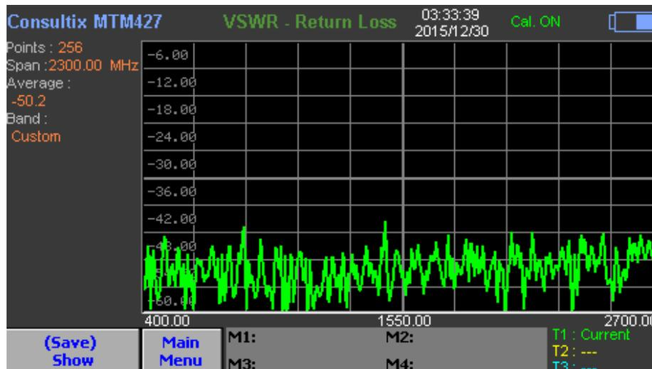
**12-**Using some quick calibration or instant calibration methods can be acceptable in some cell site troubleshooting to detect imperfection points, however a real calibration should take place to validate or qualify the installations
